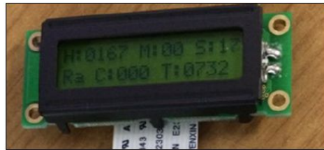
Figure 2. LCD display showing radon concentration data
